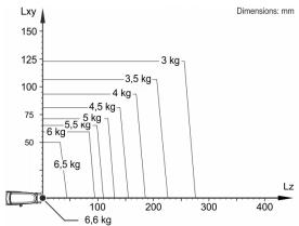
The KR 6 R700-2 is designed for a rated payload of 3 kg in order to optimize the dynamic performance of the robot. With reduced load center distances, higher loads up to the maximum payload may be used. The specific load case must be verified using KUKA.Load. For further consultation, please contact KUKA Support.
